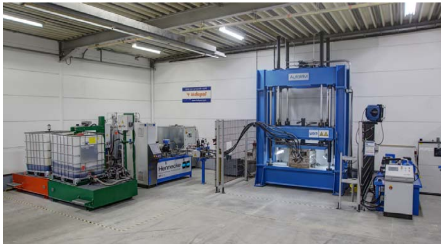
Production line – High-pressure TOPLINE HK metering machine with IBC container station and mould carrier press
