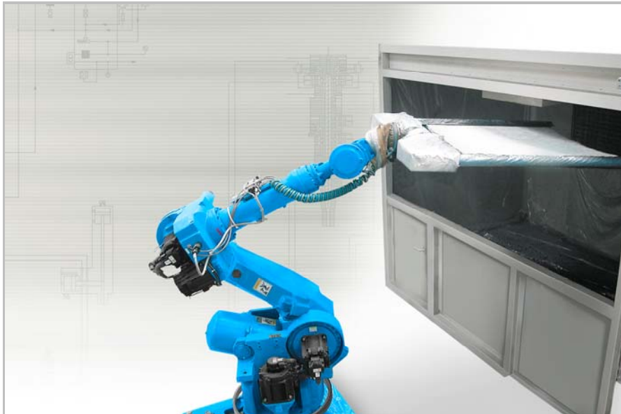
Production of a lightweight car roof with polyurethane, glass fibre and honeycomb
